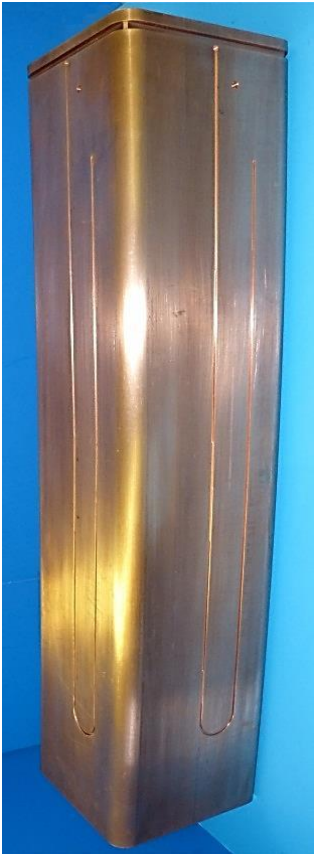
Mould tube, grooves at all four faces
